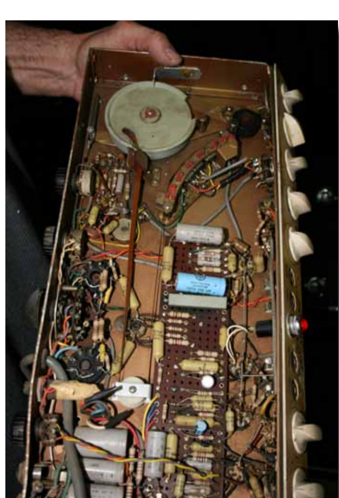
Clockwise from above left: Phil Harris with his vintage VASE Ricochet; the capston and pinch roller and playback heads; tape loop extending 2/3 of the way down the chassis; capston motor.
