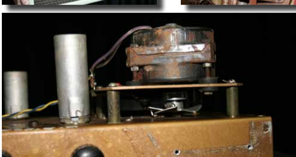
Clockwise from above left: Phil Harris with his vintage VASE Ricochet; the capston and pinch roller and playback heads; tape loop extending 2/3 of the way down the chassis; capston motor.
