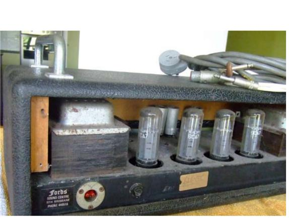
I am not sure which are the original spec! Do you know of any Vase fans that will know the tube compliment for this amp? Are there schematics out on the web? I would like to replace the electrolytic caps and check the resistors for drift/failure. Thanks, Michael
