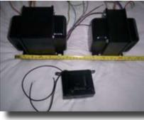
Transformers and choke have been custom wound here in Australia and these substantial components are pictured here prior to mounting in prototype.
