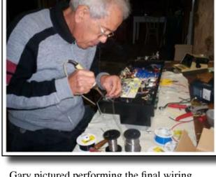
Custom wound Australian manufactured power and output transformers are mounted to chassis by Gary
